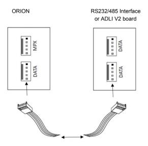
5-way flat cable from DATA 5-way connector on underside of ORION main boards to DATA 5-way connector on RS232/485 or ADLI V2 board
