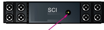
Short Circuit Indicating LED
