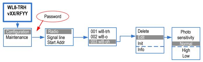
3 sensitivity options are available, these can be selected only by using the translator menu or the Ekho Configurator software (setting via the control panel will have no affect and sensor will remain in the selected mode).
