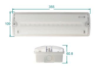
**Specification:** Weatherproof (IP65) and robust (IK10) self-contained emergency LED bulkhead. Constant emergency light (1.5W/170lm) for 3 hours. Low stand-by power consumption. Self-test versions and remote controls available. Self-adhesive legend available for 20m viewing distance exit sign. Lithium battery integrated. Maintained or non-maintainedconfigurations. Suitable for indoor and outdoor applications such as car parks, distribution centres, storage rooms and sports centres.
