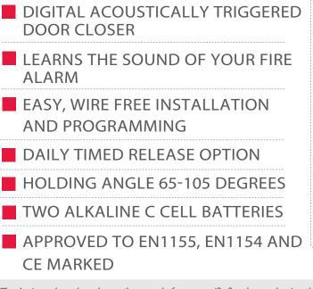
The Agrippa door closer learns the sound of your specific fire alarm, releasing the door in the event of a fire.
