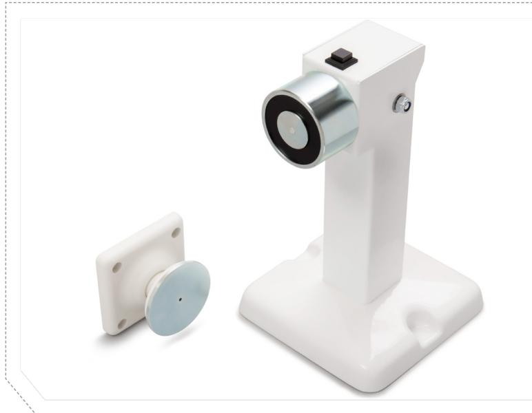
This rugged, versatile design of door magnet can be used for many different door holding applications. With the magnet set as shown in the photograph, the door holder can be floor mounted or ceiling mounted. Turn the magnet through 90° and the door holder is in wall mounting configuration.
